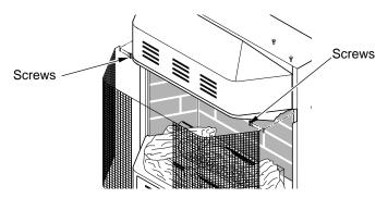
Figure 11 - Removing Screen
